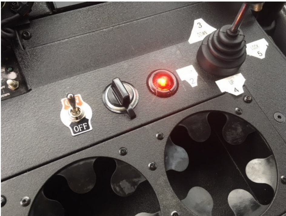
Joy Stick operated from within the cab
